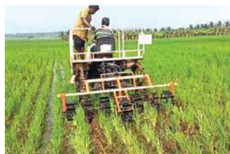
Multi-row rotary weeder attachment to rice transplanter
