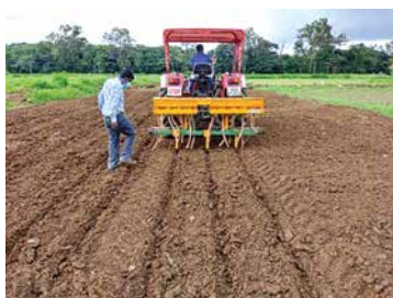
Micro-controller based precision planter for maize and cotton
