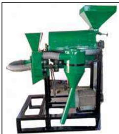
Small millets dehuller (Abrasive type)
