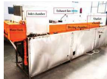
Refractance Window (RW) drying based fruit bar manufacturing system
