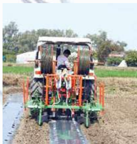
Drip lateral and plastic mulch layer-cum-planter
