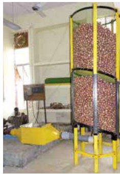
Modular onion storage structure
