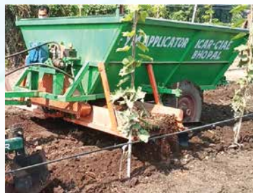
Trencher-cum-FYM applicator for grape orchards
