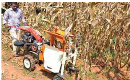
Self-propelled small maize harvester
