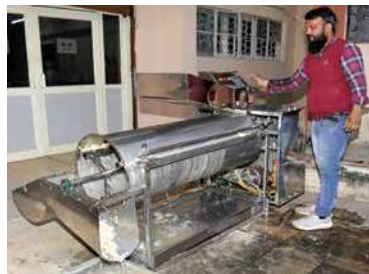
Peeling machine for medicinal root crops
