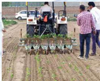
Tractor operated Paper-tape Vegetable Transplanter
