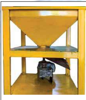
Rotating orifice feeding system for makhana popping machine
