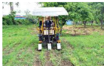
Solar assisted e-prime mover for field operations
