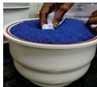
Seed desiccation over charged silica gel
